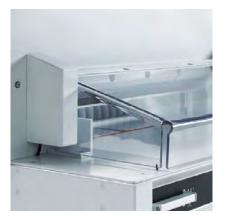
TRANSPARENT SAFETY GUARD A cut can only be executed, if the hinged, electronically secured safety guard on the front table is closed.
